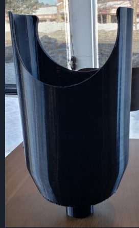
Figure 18: 3D printed supporting channel
