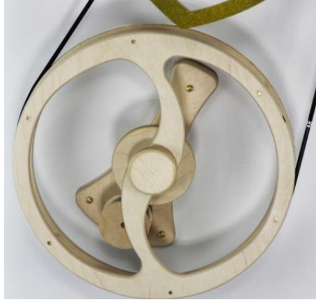
Figure 3.4.1.3b: Close-up of Circumvolve's winding mechanism [7]
