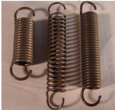
Figure 7: Helical Back Springs
