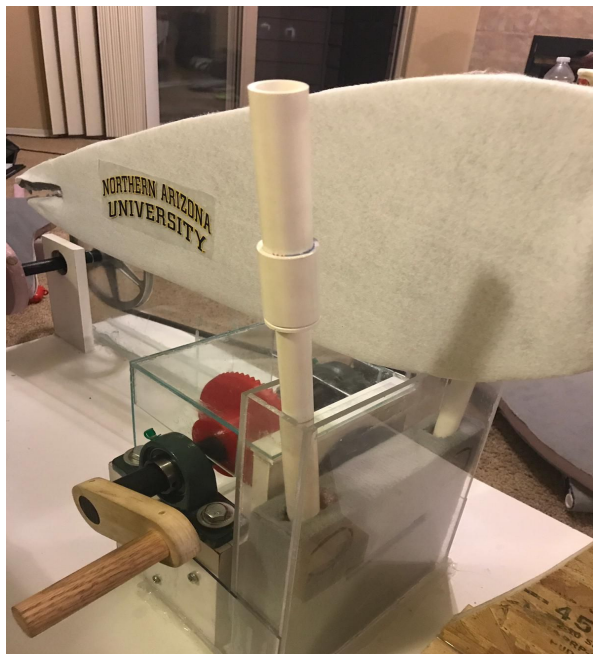
Figure 14: Right plastic PEX rod part #2
