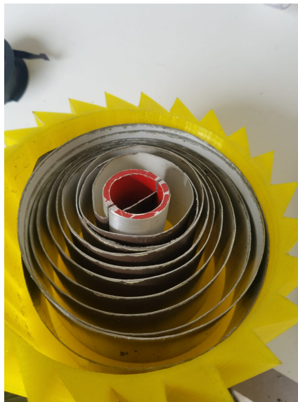
Figure 2: Ratchet gear and it's spring
