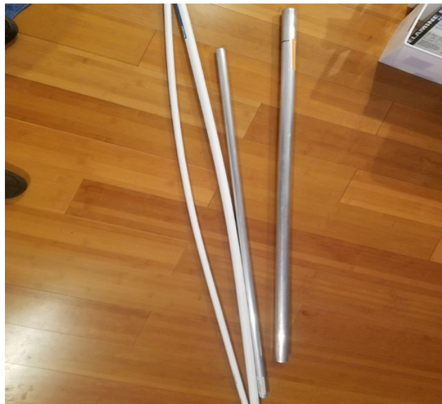
Figure 3: Metal pipes that will be used for shafts along with plastic PEX pipes that will be used to create the hinge for the wings.
