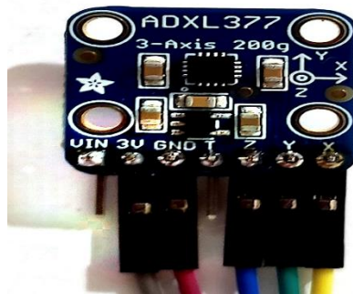
Figure 26: Triple-Axis Accelerometer (+-200g)
