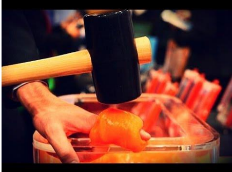
Figure 9: D30 Material Protecting Hand from Hammer
