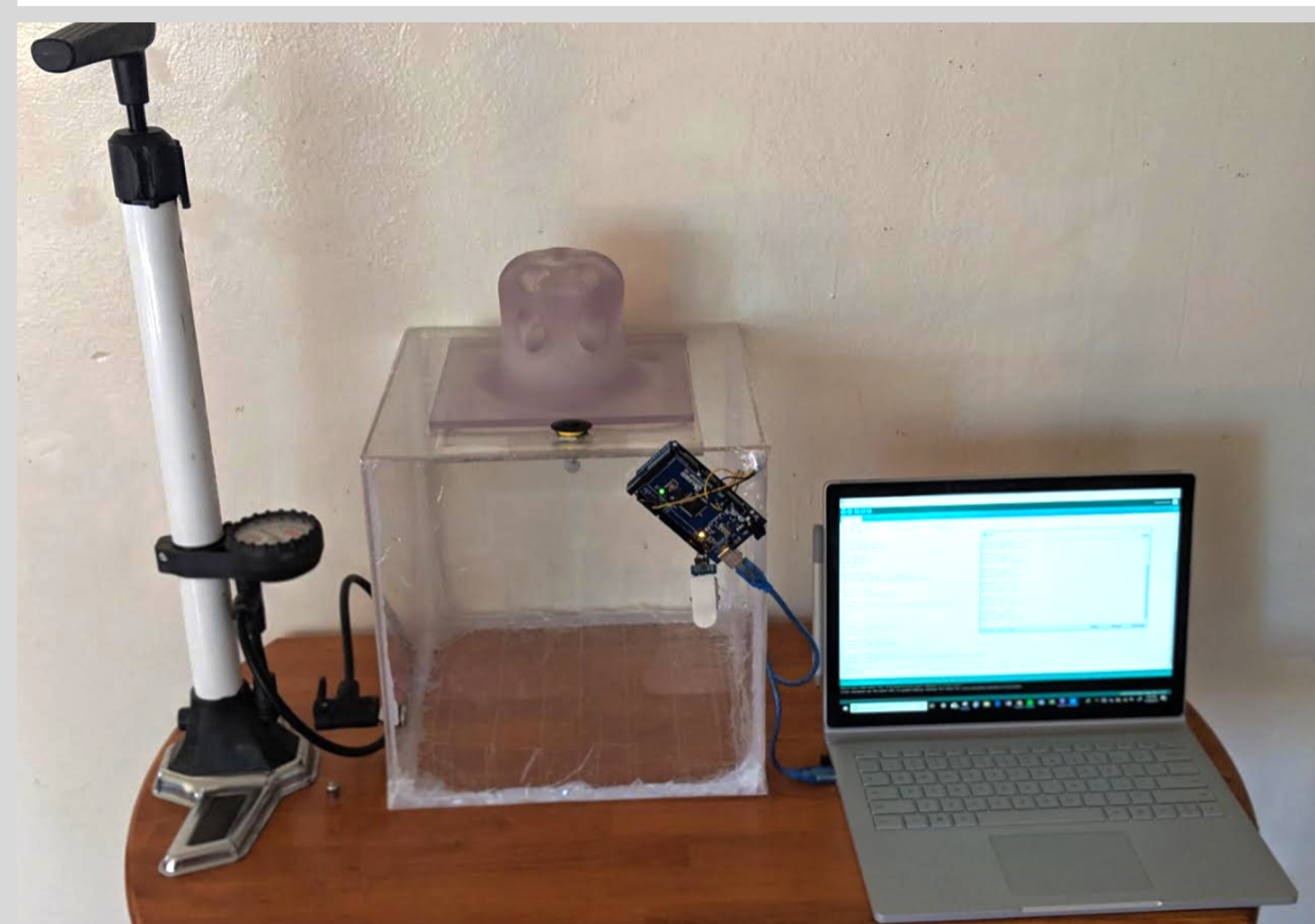
Figure 7: Test Setup with Termite Vent in Test Position
