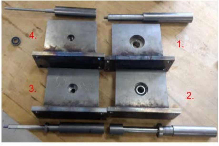
Figure 17: Shafts and Bearing Housings
