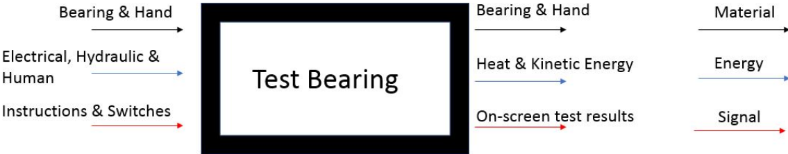
Figure 3: Black Box model for Testing Bearing
