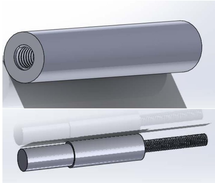
Figure 25: Initial Threaded Shaft Design
