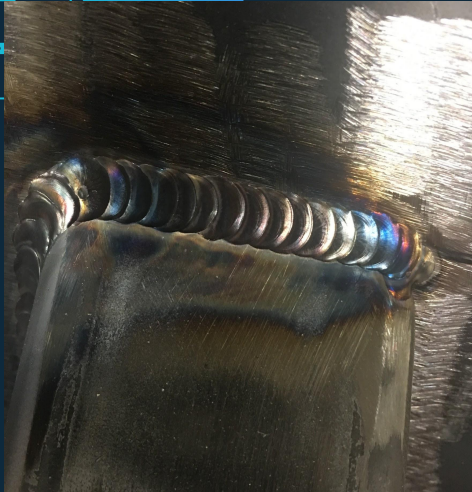
Figure 23: Truss Fillet Weld
