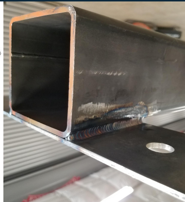
Figure 7: Steel Plate Weld
