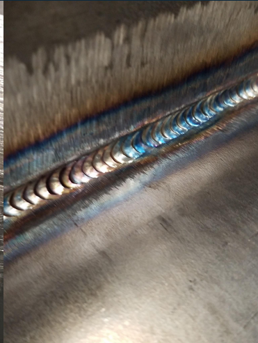
Figure 24: Cross Beam Fillet Weld
