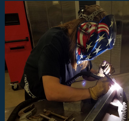
Figure 22: Welding Truss Plate
