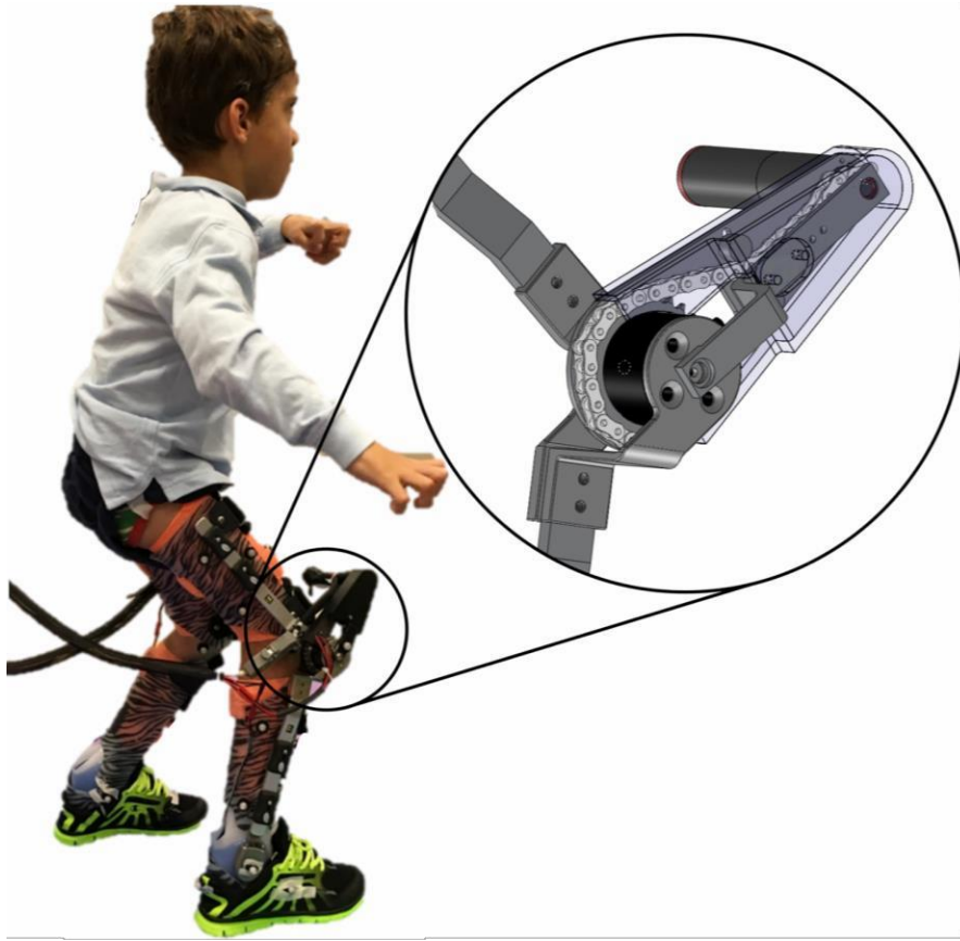
Figure 1. Exoskeleton mounted to custom-molded orthotic
