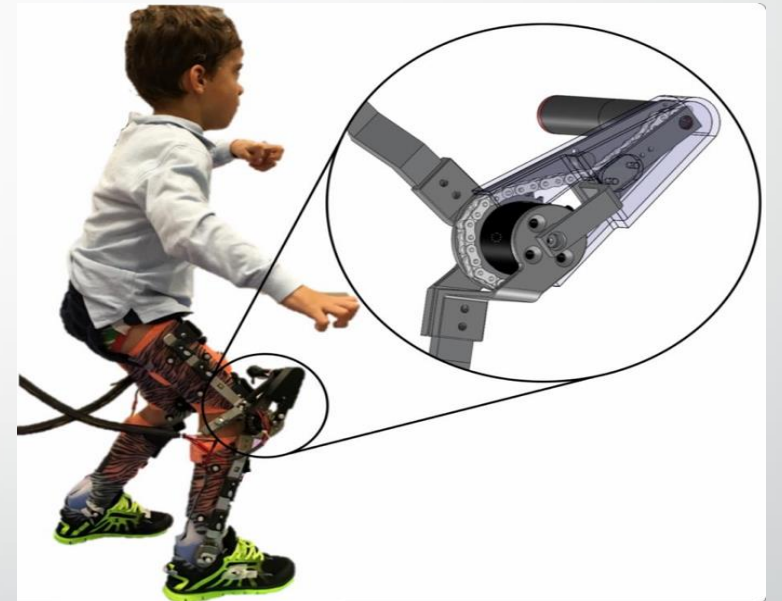
Figure 1: Adjustable Human-Exoskeleton Mounting Interface
