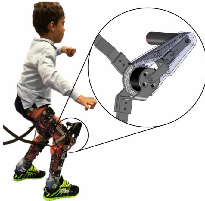
Figure 1. Adjustable Human-Exoskeleton Mounting Interface [1]
