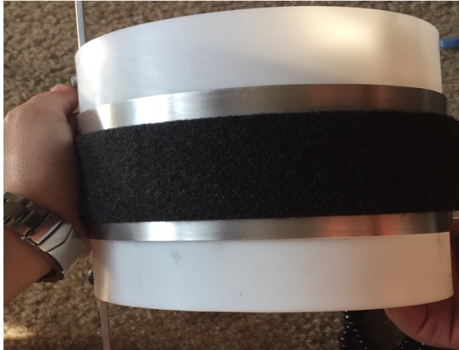
Figure 38. Thigh Area with Velcro Tape and Aluminum Sheet.
