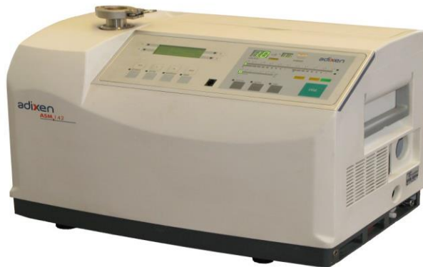
Figure 6: Helium Leak Detection Machine
