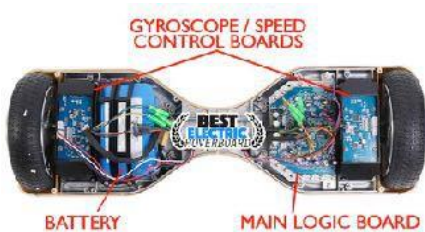
Figure 27: Hover Board Main Parts [17]
