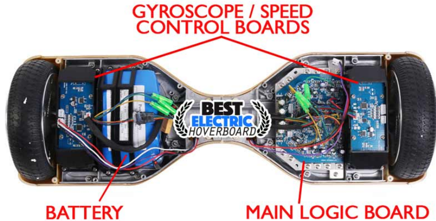
Figure 27: Hover Board Main Parts [17]
