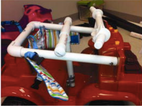
Figure 3 Roll cage on a ride-on-car with PVC pipes
