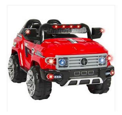
Vehicle used as base design Initial Features: (2) 12 V Motors Variable speed control (2 mph & 4 mph) Forward and reverse control Seat belt Operated through foot pedal or remote control
