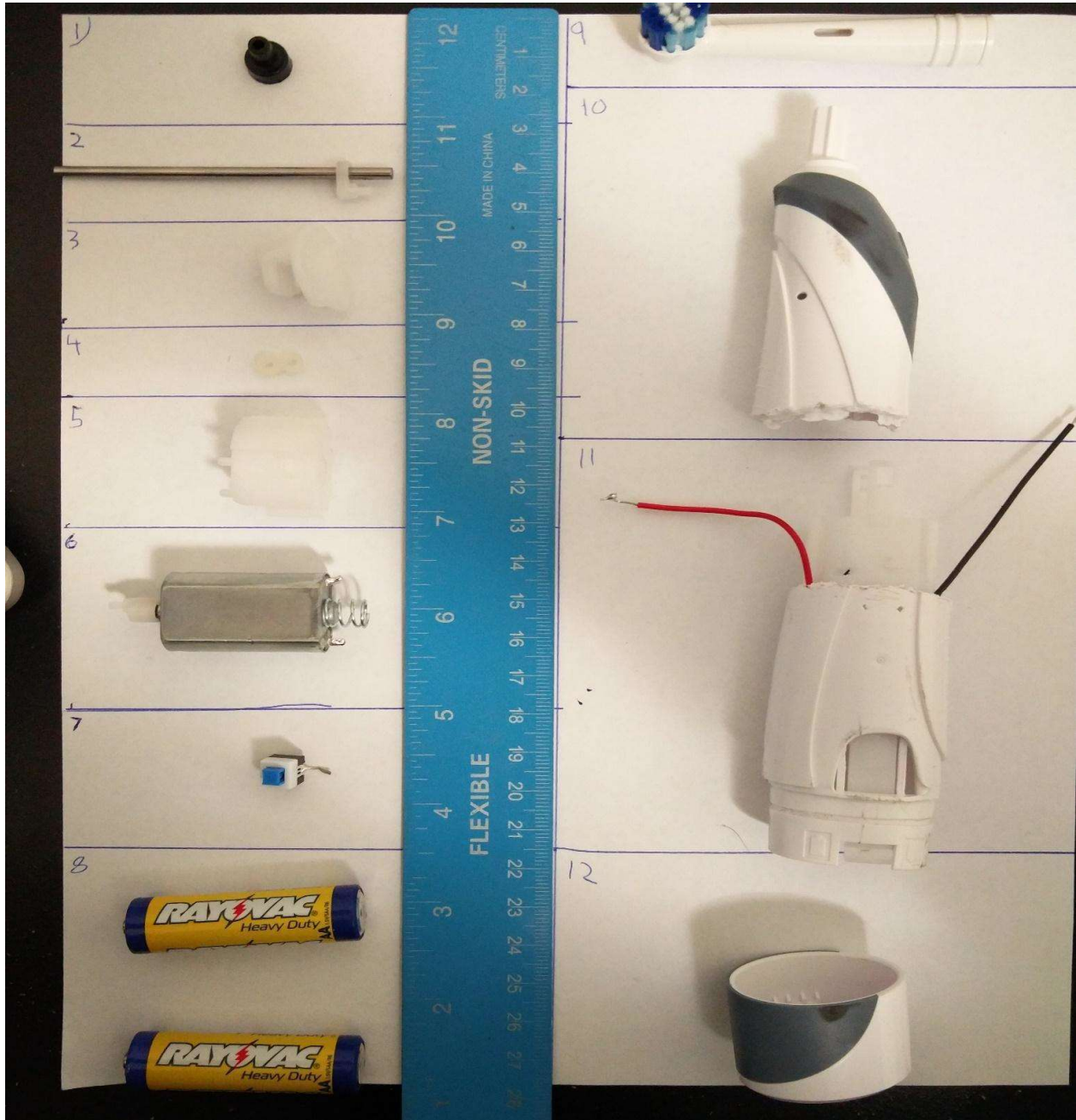
Figure 3: Electric Toothbrush parts
