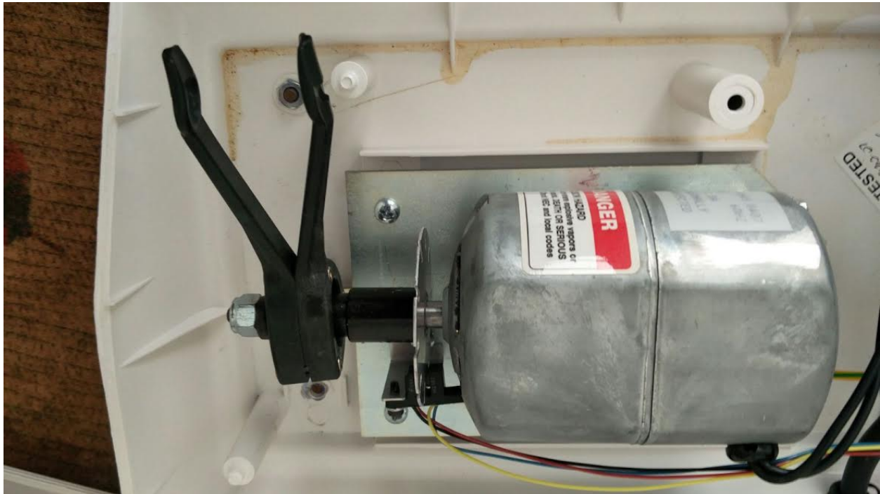
Figure 1: Original Dental Triturator Components
