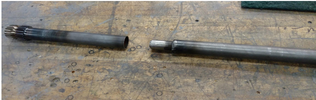
Broken Steering Shaft
