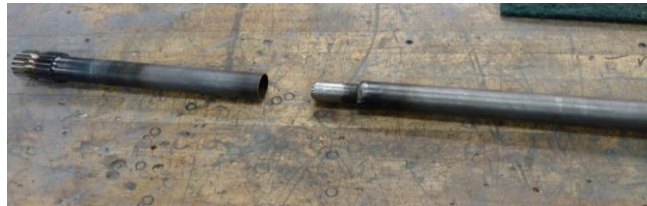
Figure 30: Broken Steering Shaft
