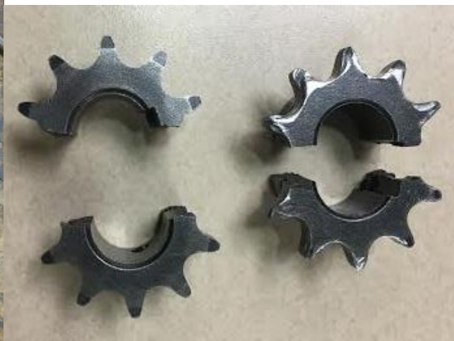
Figure 34: Second Broken Chain Sprocket
