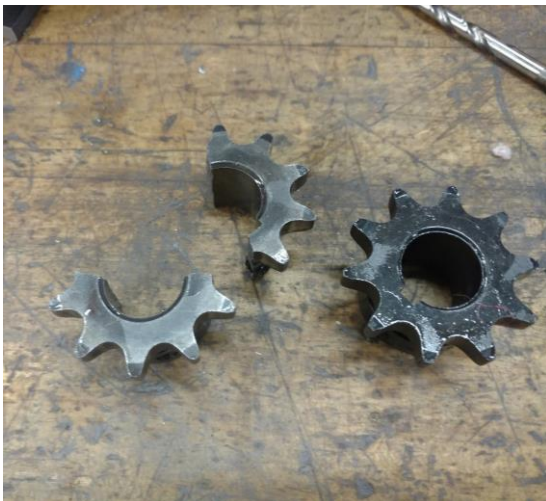
Figure 33: First Broken Chain Sprocket
