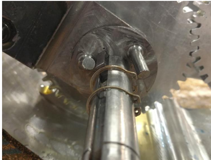
Figure 35: Bent Engagement Pins
