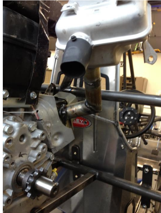
Figure 2: Old Muffler Front View
