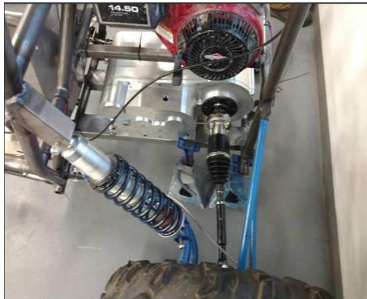
Figure 10: Three-link Rear Suspension
