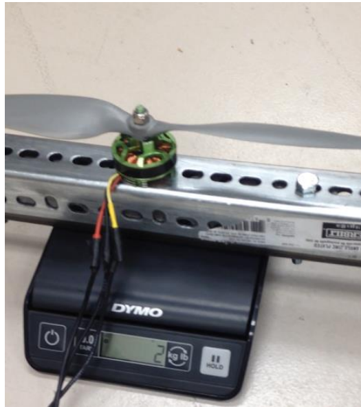
Figure 31 – Thrust test setup.
