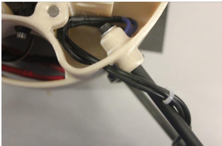
Figure 29 – Boom attachment setup
