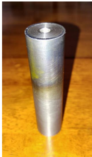
Figure 8: Front iron end cap heat-fitted in solenoid casing
