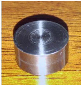
Figure 6: Steel impact plate
