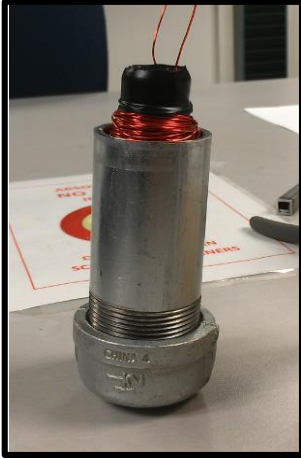
Figure 1: Proof of concept for the solenoid (left) and micromotion (right)
