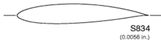
Figure 5: geometry for airfoil S834 with error in inches [5]
