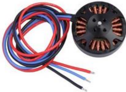
Figure 13: SunnySky X4130S 480kv brushless motor [12]
