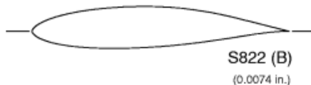
Figure 4: geometry for airfoil S822 with average error in inches [5]
