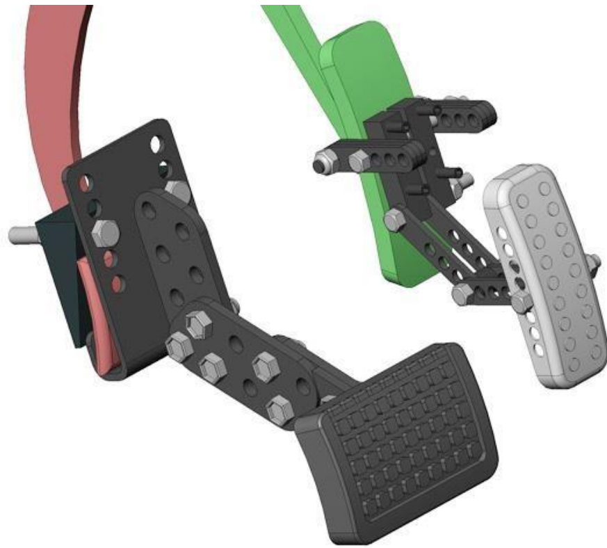
Figure 13: 3-D Model of Off-the-Shelf Foot Pedal [1]
