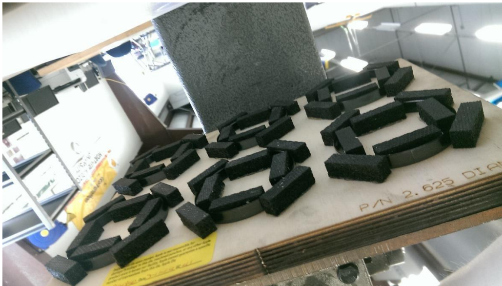
Figure 6: Cutting Press Blades (with foam guards)
