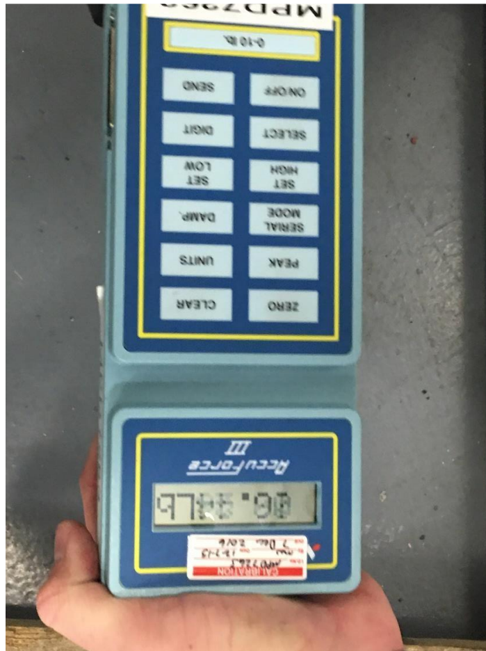
Figure 53: Force Gauge Display, Foot Lever w/o Extension
