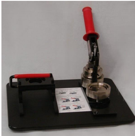
Figure 7: Tecre Mounted Manual Button Maker
