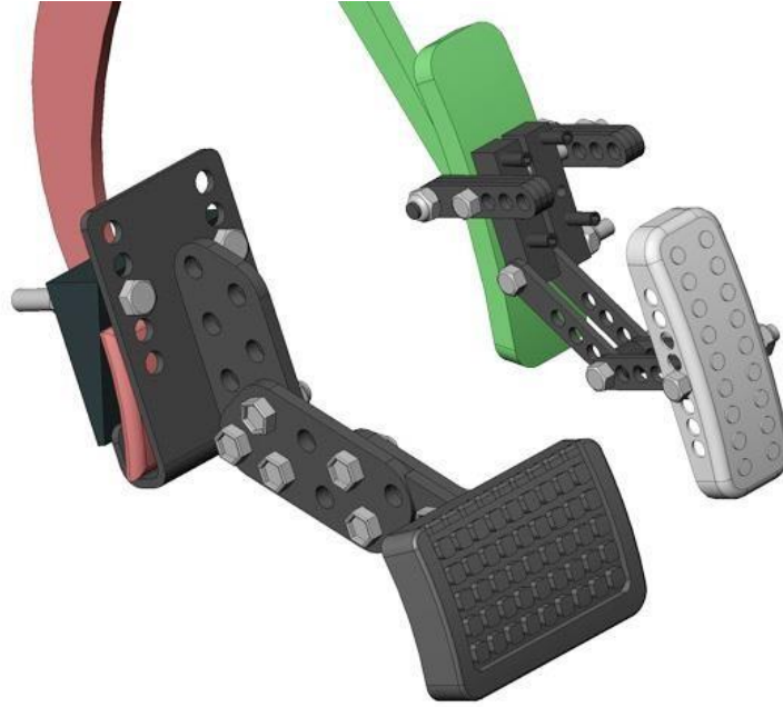
Figure 50: Foot Pedal Extension Installed on Foot Lever[12]
