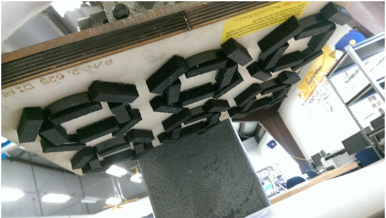
Figure 49: Steel Blades (6) mounted on Upper Plate
