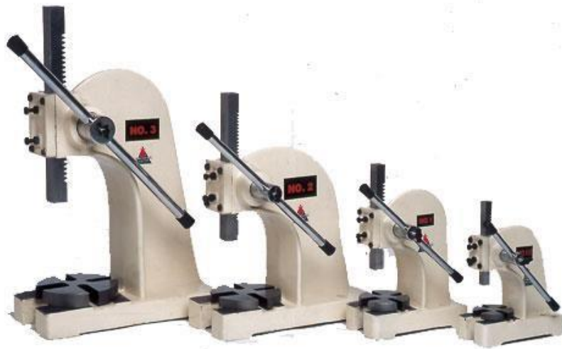
Figure 20: Arbor Press to be Modified[11]
