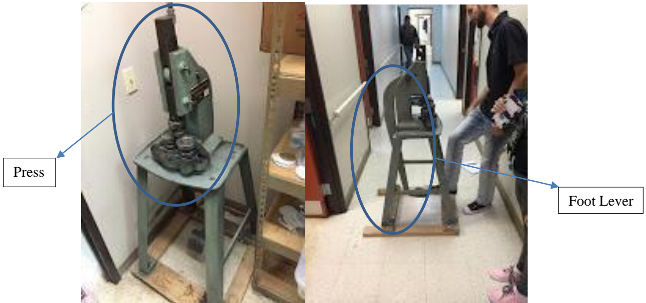
Figure 3: Button Maker Press
