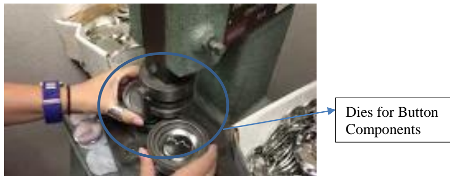
Figure 5: Button Maker Dies
