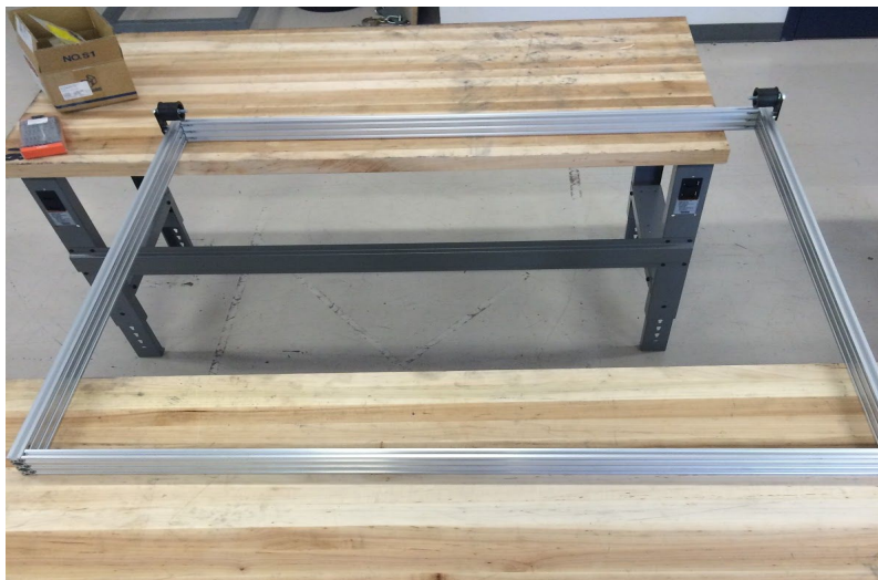
Figure 10.8 - Gantry Rail Setup
