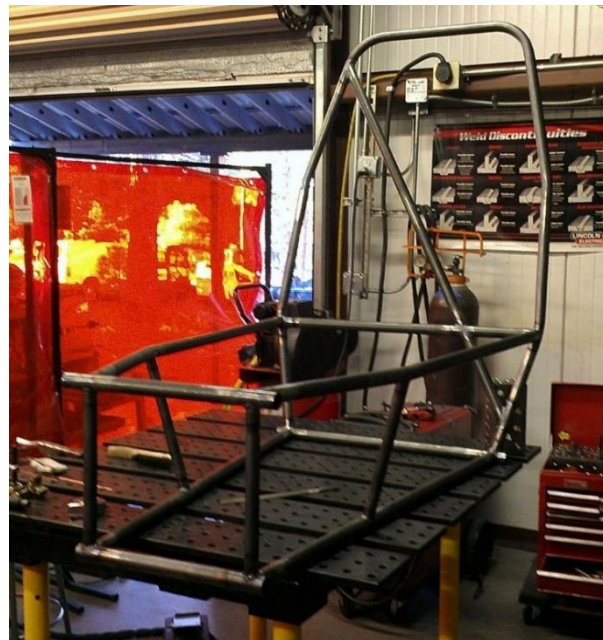
Figure 19: Diagonal Supports and SIM support added to the Frame.
