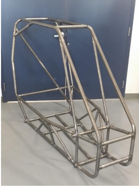
Figure 5: Current Frame Progress.
