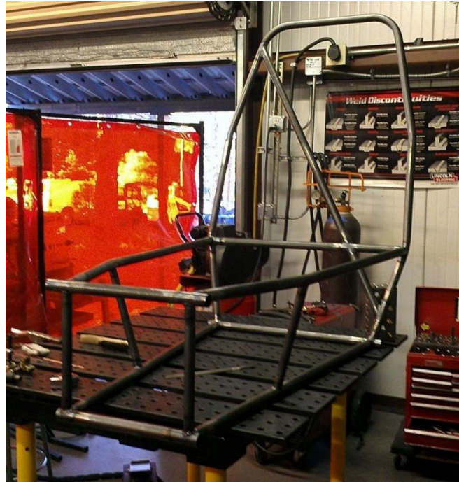
Figure 4: Diagonal Supports and SIM support added to the Frame.
