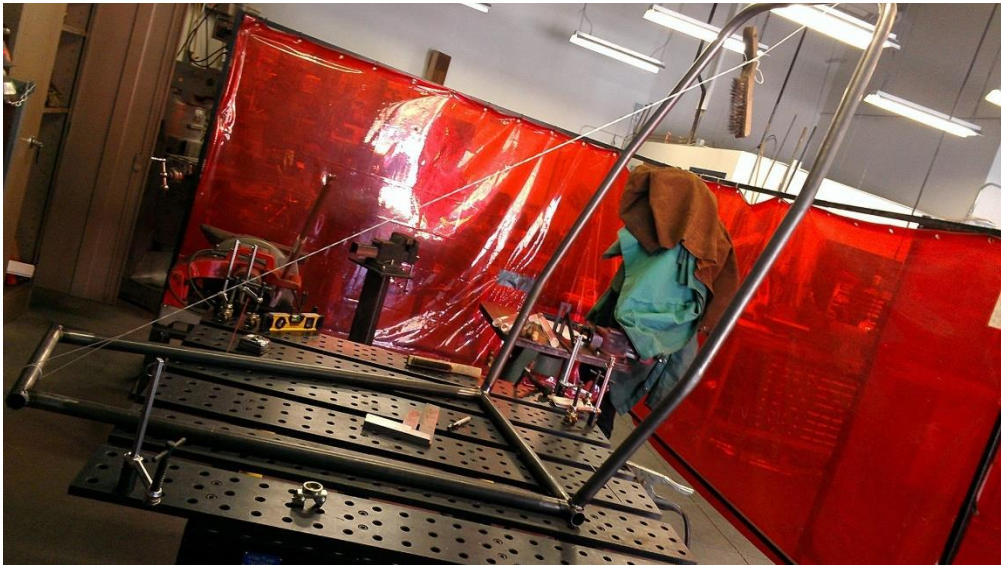
Figure 2: Firewall about to be TIG welded to the bottom Supporting Members
