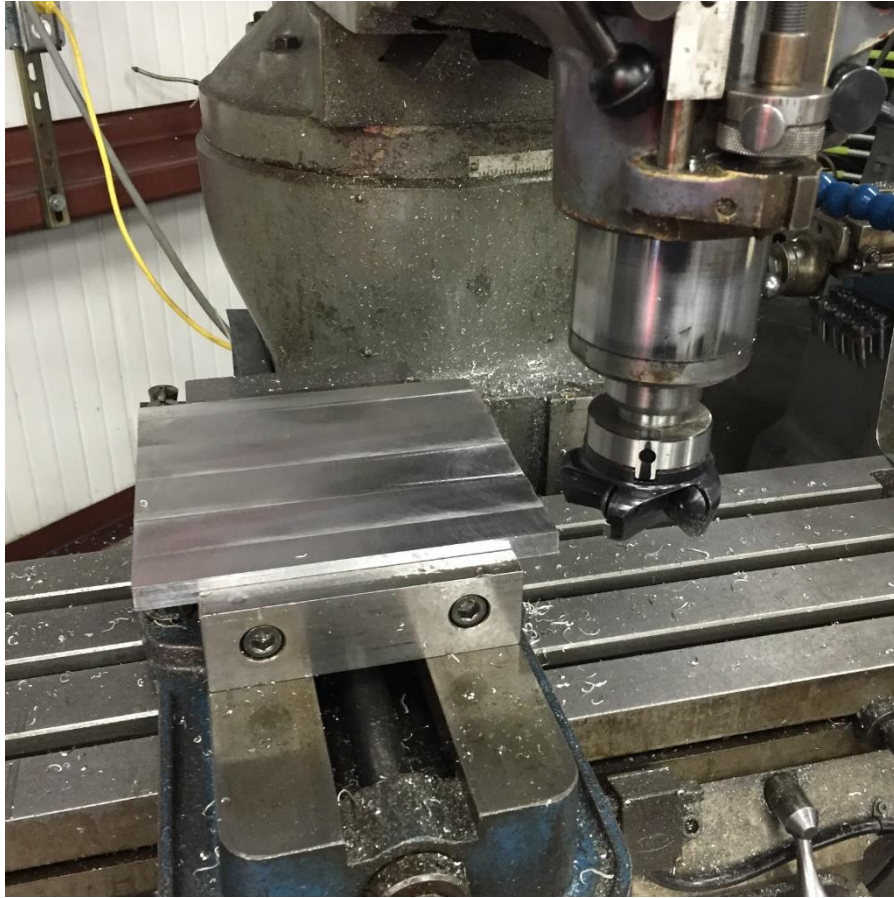
(Figure 4.1, Facing Aluminum Plates)
