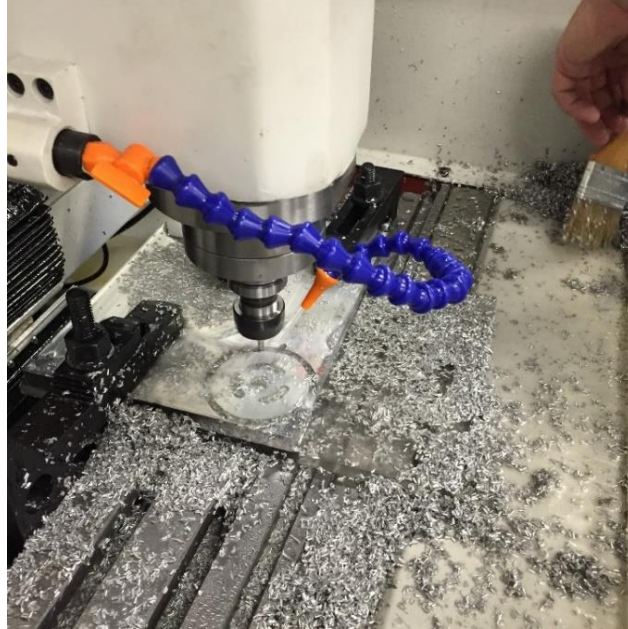
(Figure 4.2, Cutting out Gear Blanks)
