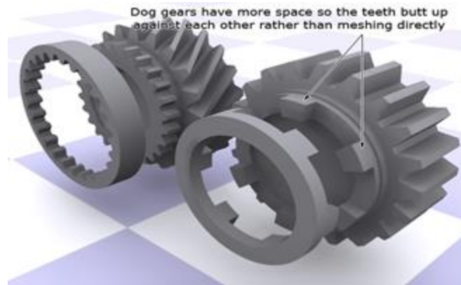
(Figure 2.1, Manual (left) Vs. Sequential (right) dog ring [1])
