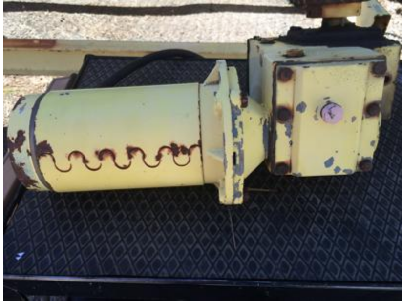
Figure 3: Motor connected to the upper level gearbox
