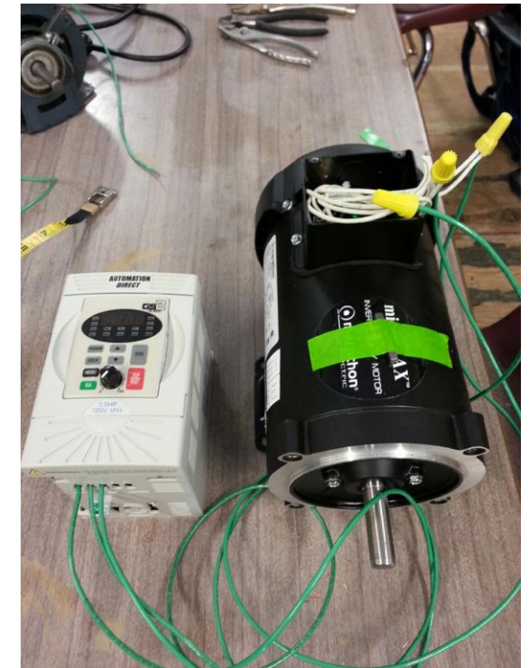
Left: Shows the connections for the motor. Right: 12 AWG wire connecting the motor to the control box.
