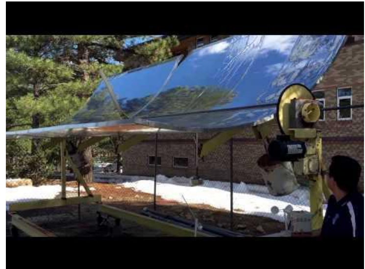
Video 3: Testing of trough rotation (CW)
