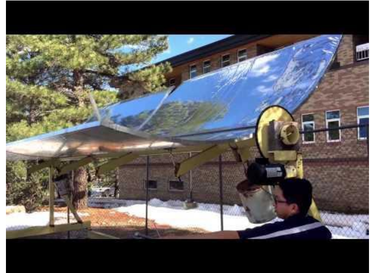
Video 2: Testing of trough rotation (CCW)
