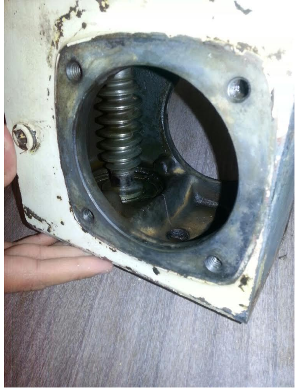
Figure 6- Lower gearbox before (left) and after (right) cleaning
