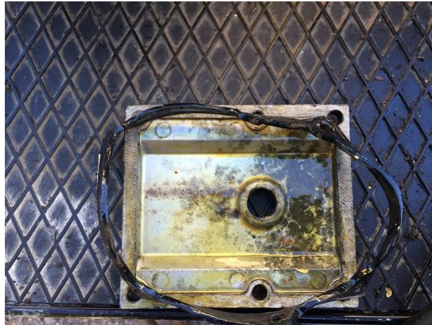
Figure 12: Upper gearbox cover
