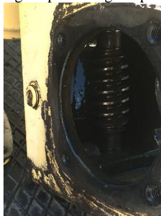
Figure 13- Vertical worm gear connecting the upper level to the lower level gearbox.
