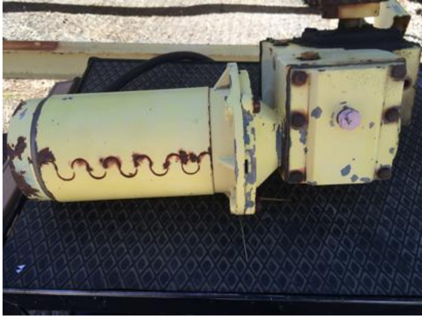
Figure 10- Motor connected to the upper level gearbox
