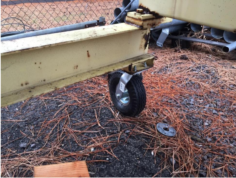
Figure 8- Replaced Caster with the tire
