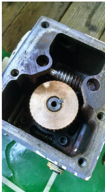
Figure 15- Post-cleaning upper gearbox
