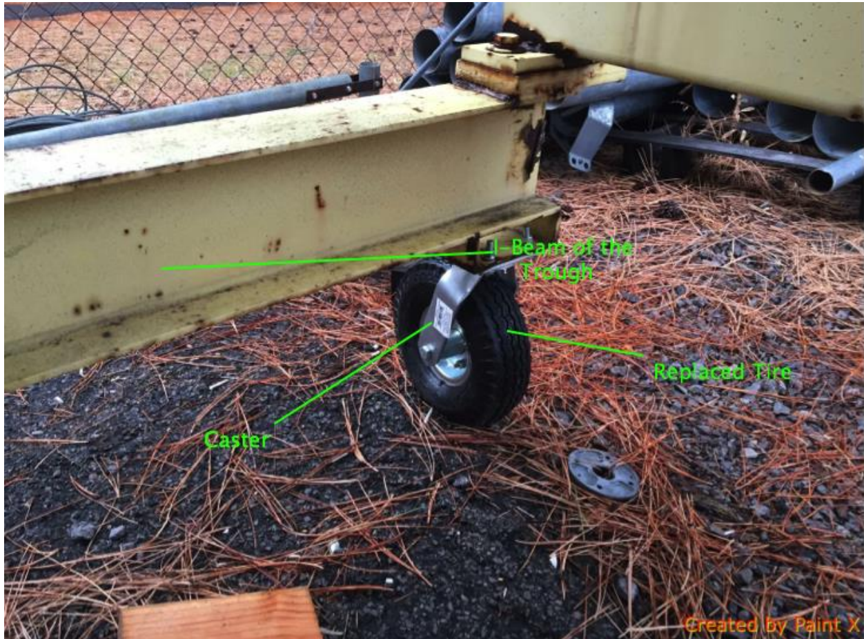
Figure 3 - Replaced Caster with the tire
