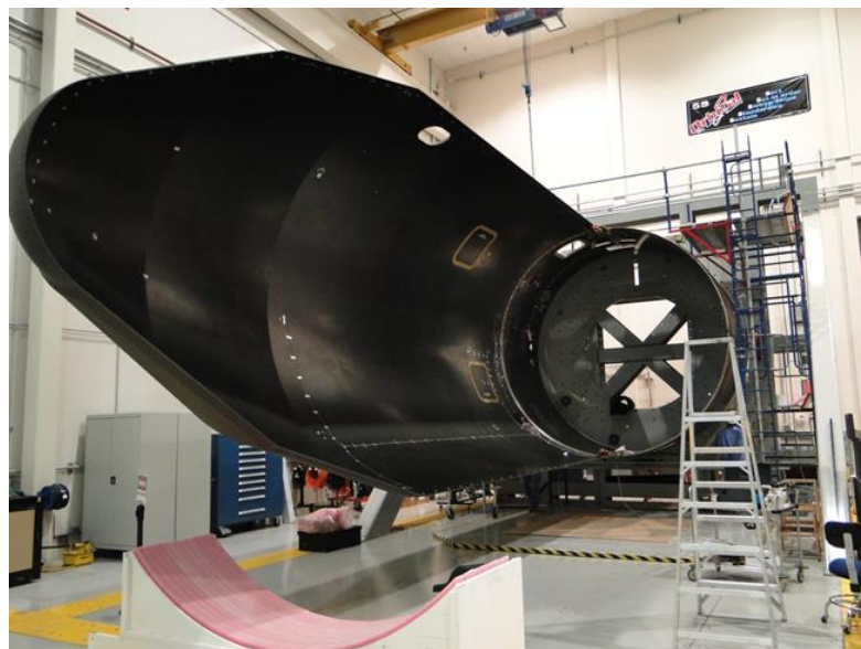
Figure 1: View of the horizontal test stand with one payload fairing loaded onto the test stand.
