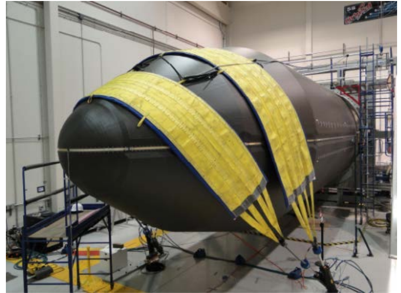
Antares launch vehicle in horizontal testing position
