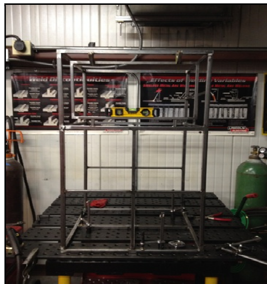
Figure 2: Frame with members welded
