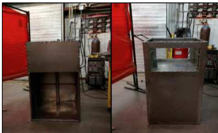
Figure 4: Front and side view of the cart with the sheet metal welded
