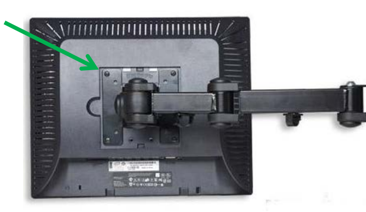
Figure 8: Hole Alignment for Mounting Monitors
