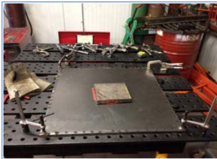
Figure 24 : Welding sheet metal
