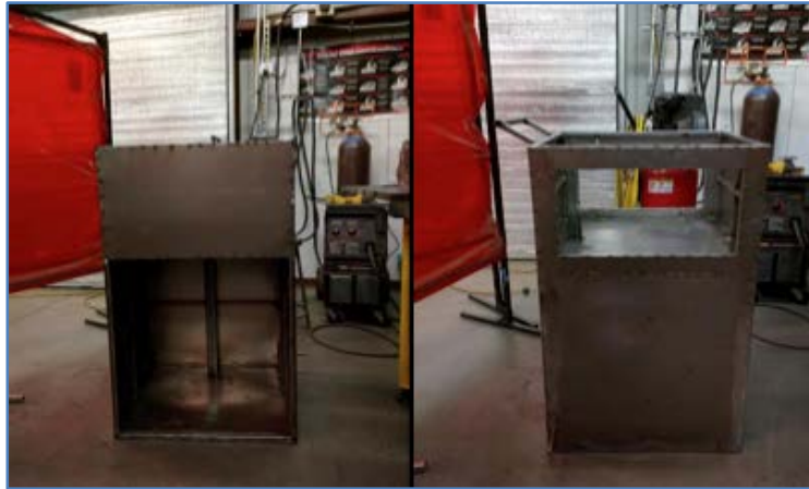
Figure 25: Front and side view of the cart with the sheet metal welded
