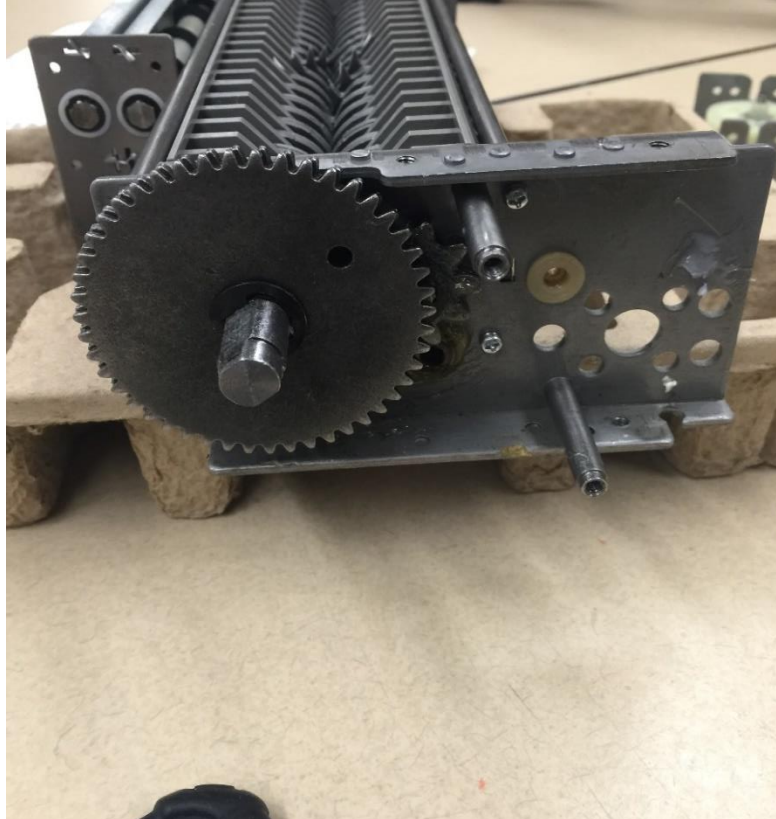
Figure 3: Internal Shredder Mechanism and Main Shaft
