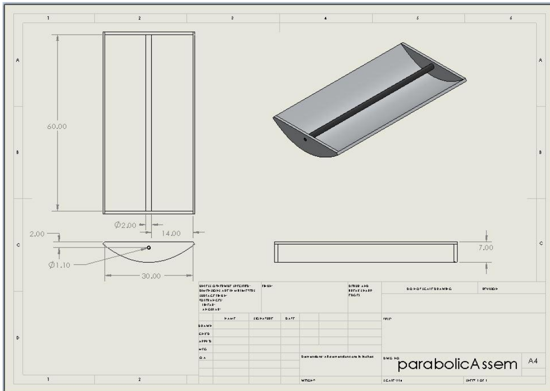
Figure 2: Parabolic collector engineering drawing.
