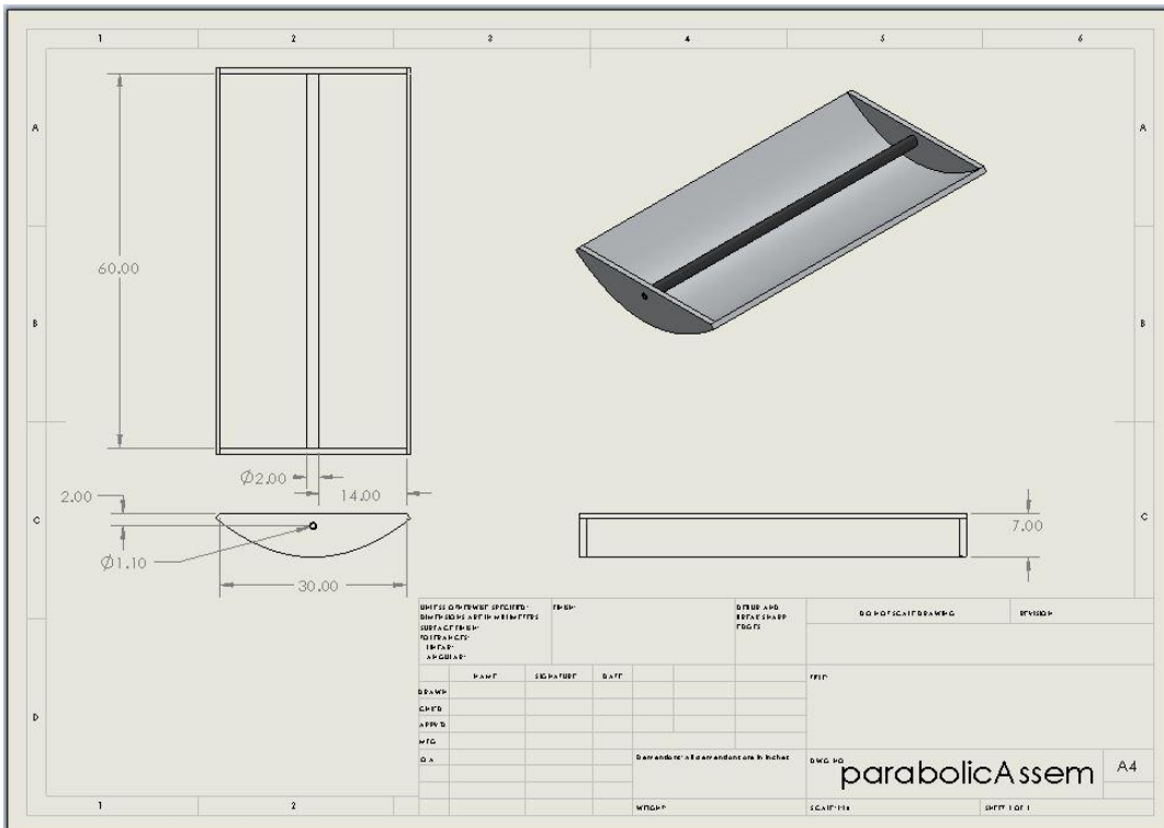
Figure 2: Parabolic collector engineering drawing.
