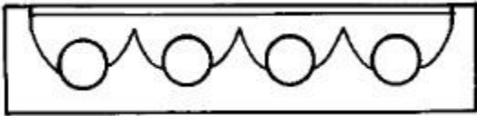
Figure 2: Parabolic Crescent Collector
