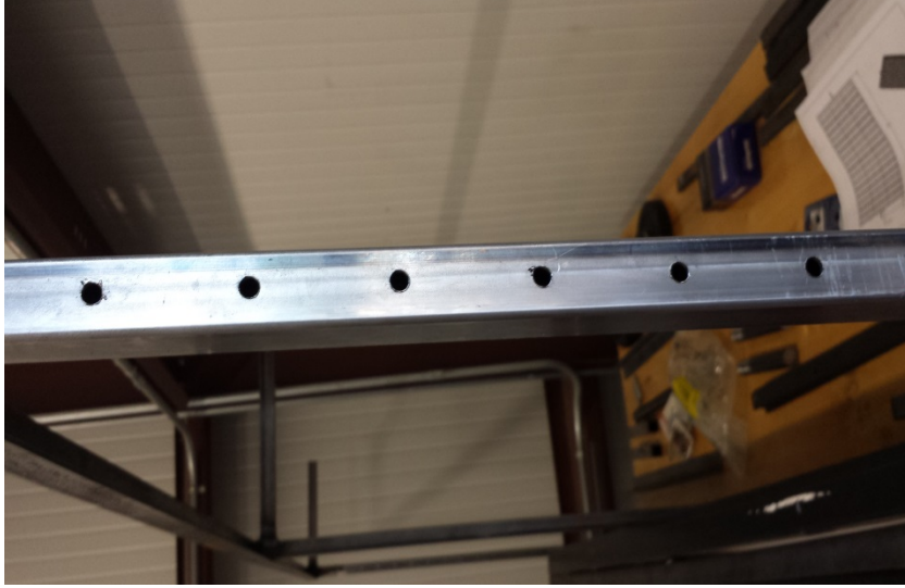
Figure 4: Holes for manual North-South tracking
