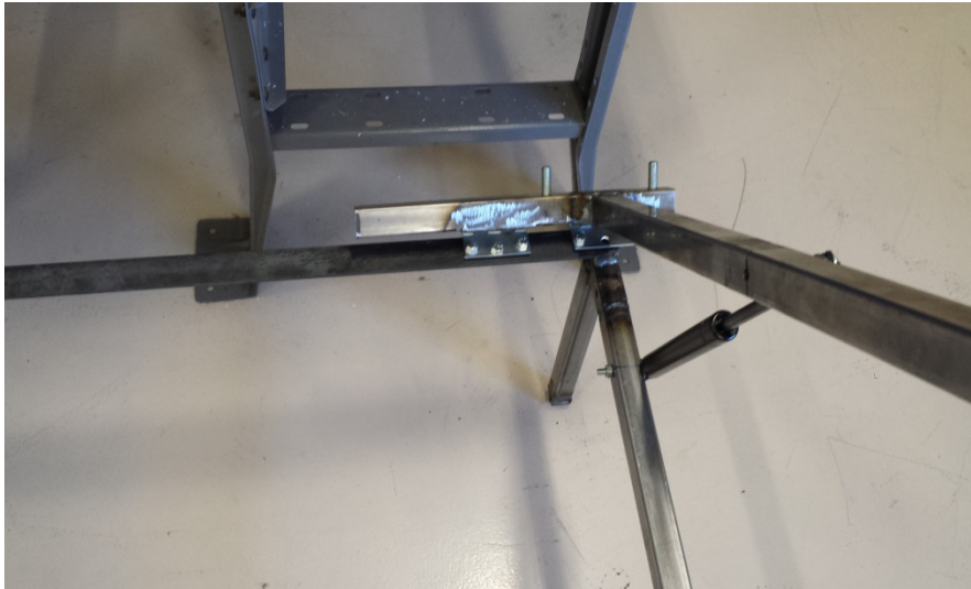
Figure 3: Connections of base frame and angle support
