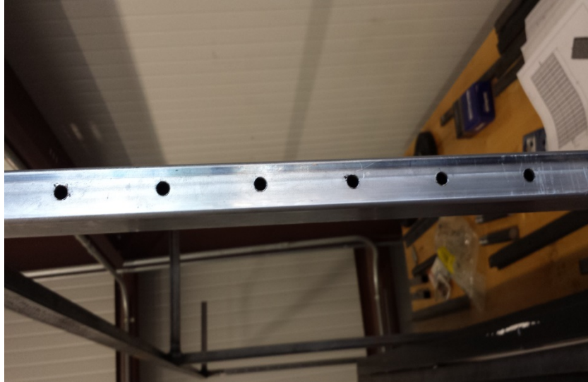
Figure 7: Holes for manual North-South tracking
