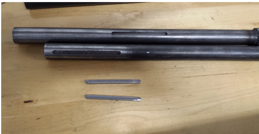
Figure 15: Keyways and key
